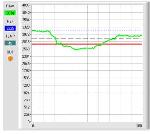
When the current measurement value **RAW** (green line) rises above the hysteresis threshold (black line) again, the output **DIGITAL OUT** changes to +24V again (signal is OK). This is visualised by the **OUT** LED.
