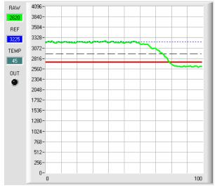
When the current measurement value **RAW** (green line) falls below the switching threshold (red line), the output **DIGITAL OUT** changes to 0V (error). This is visualised by the **OUT** LED.
